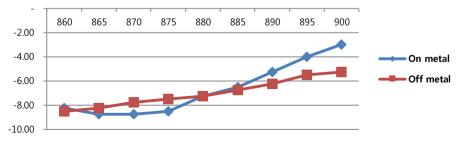
•Fastener TK reads 10% shorter off metal (or on non metal surface). It can be applied for BOTH metal and off metal application.
