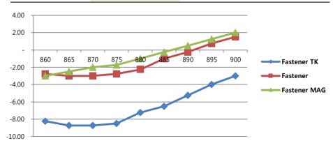
•Fastener TK reads up to 12.0 meters on metal, almost double of Fastener and 50% longer than Fastener MAG. It's one of best performing among 4mm thick metal tags with most stable and consistent read, as its flat and gentle slope of sensitivity curve shows.
