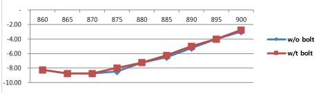
•Fastener TK reads same, regardless of whether it is fastened with metal bolt in two holes (located on center of both ends) or not. Stainless steel M4 bolt with round head is best fit for Fastener.
